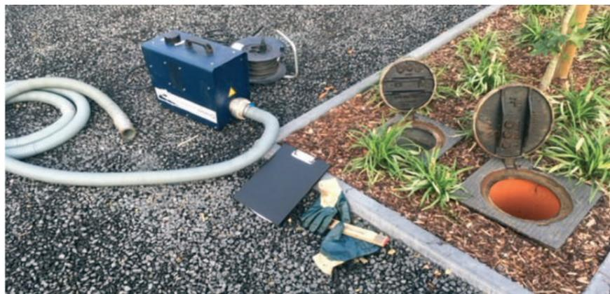
Picture 1: Testing of private sewer connections
