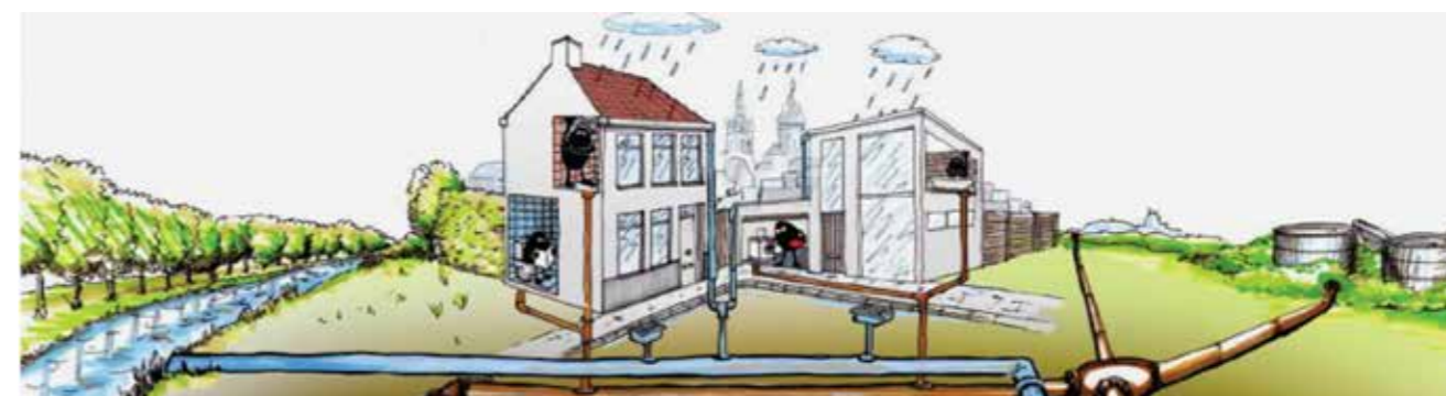
Picture 2: Connections on separate sewer system
